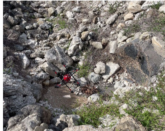
Fig. 11: 4-Gas PLUS sensor in drainage ditch to monitor for run-off
