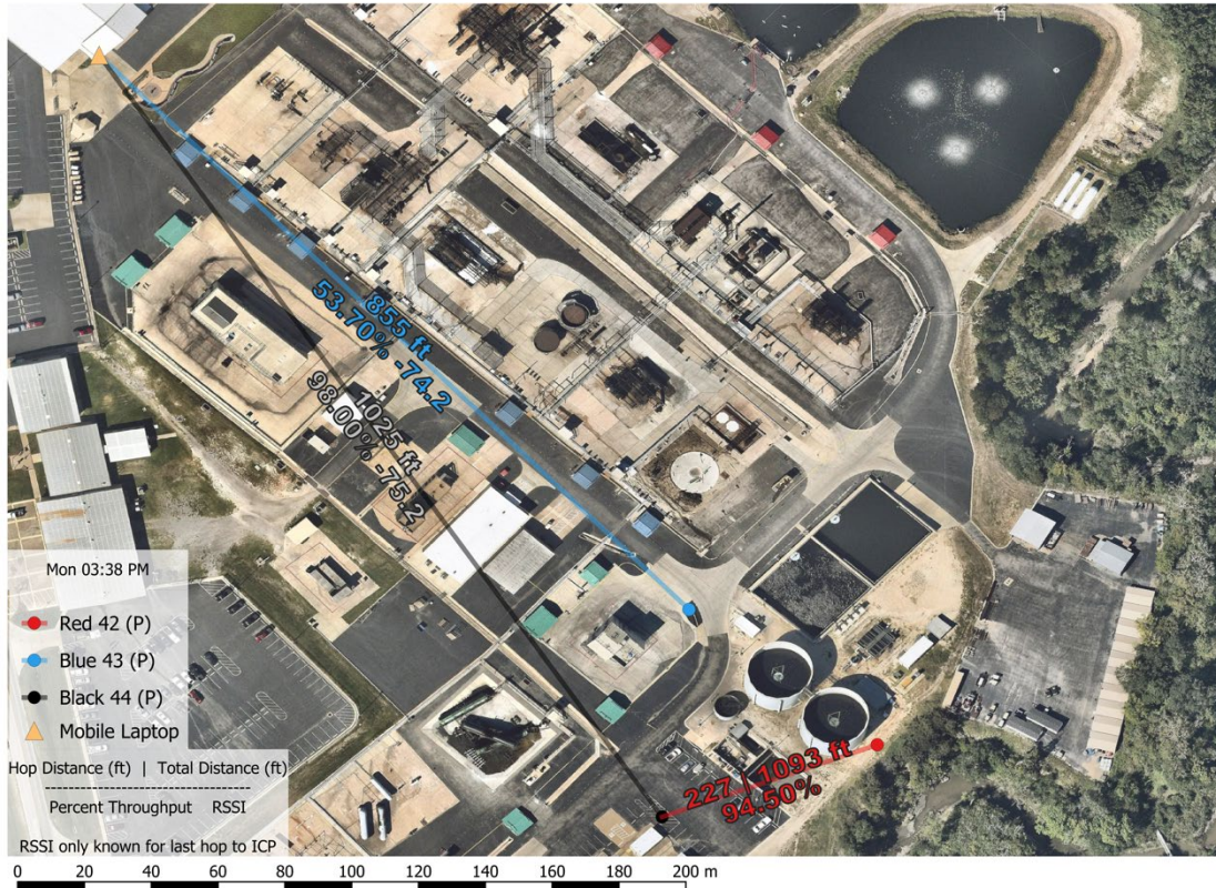
Fig. 22: Longest transmission range of 1093 ft recorded at Bulk Storage Tanks prop (indicated in bold italic in table); achieved through 1-hop mesh
