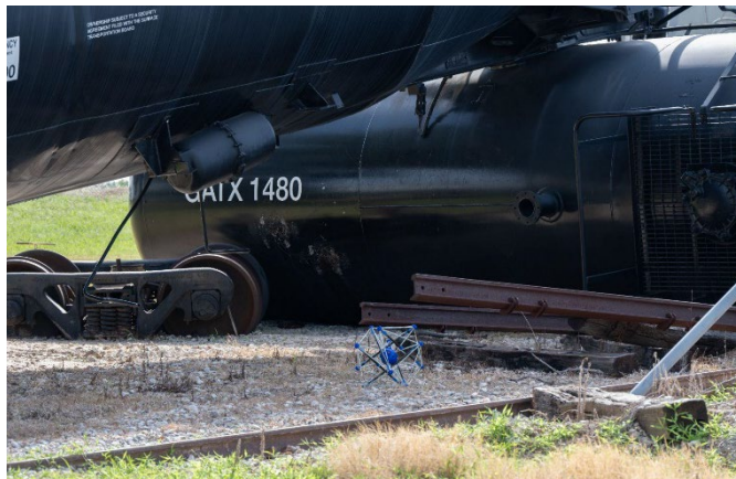
Fig. 10: 4-Gas PLUS sensor placed near identified potential leak site
