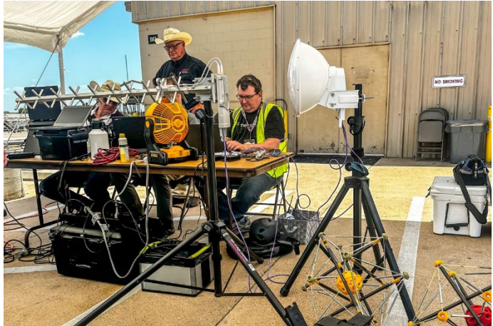
Fig. 21: RF interference data collection set-up at water tank storage testing prop
