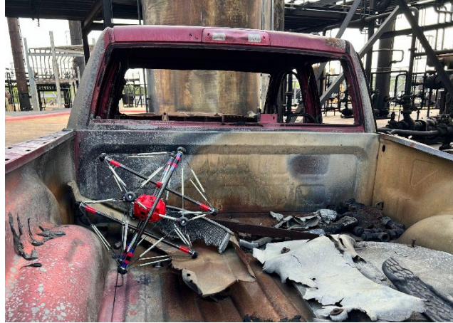
Fig. 16: 4-Gas PLUS sensor strategically placed in location surrounded by metal
