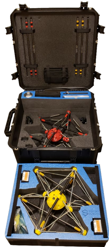
Figure 1 Two Squishy Robotics Stationary Robots, one Custom payload, and 4-Gas PLUS Sensor payload packed in hard shipping case.
