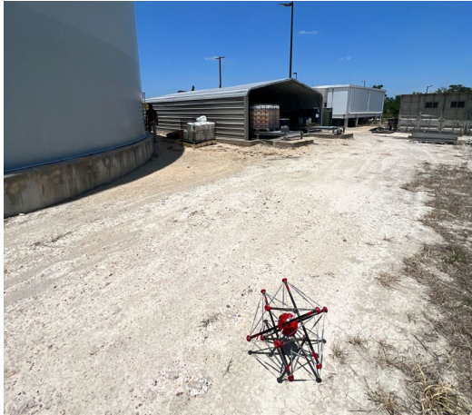
Fig. 20: 4-Gas PLUS sensor deployed behind water storage tank
