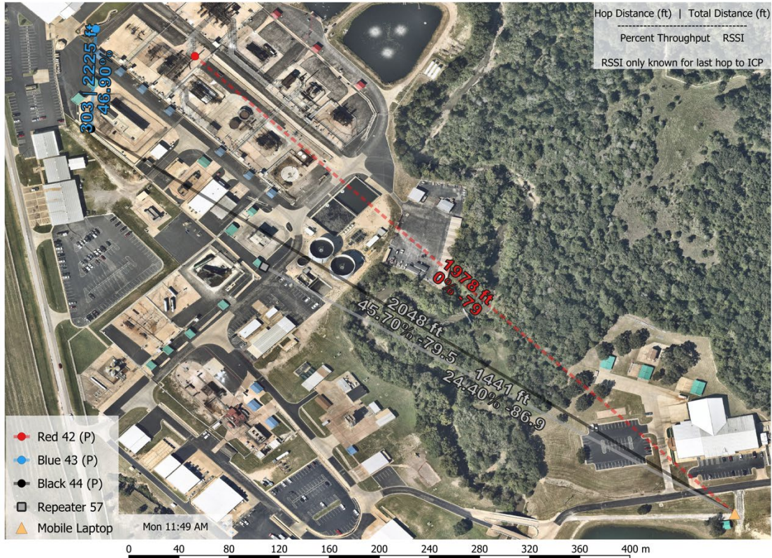
Fig. 17: Longest transmission range of 2225 ft recorded at petro/chemical plant testing prop (indicated in bold italic in table); achieved through 1-hop mesh
