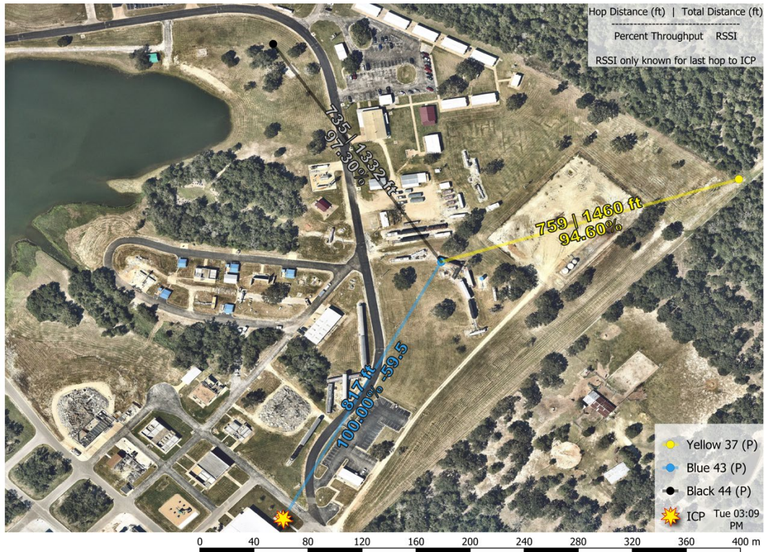
Fig. 12: Longest transmission range of 1460 ft recorded at Train Derailment prop (indicated in bold italic in table); achieved through 1-hop mesh
